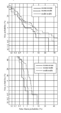
Fig. 1. DET plot for Z-NORM a posteriori (top) and U-NORM (bottom) techniques in three different training and testing conditions
