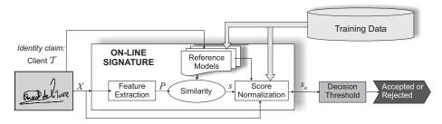
Fig. 1. System model of biometric authentication with score normalization
