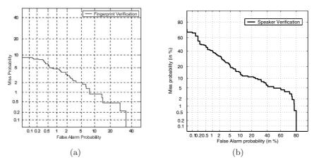
**Fig. 2.** DET curve of: (a) ATVS reference fingerprint system with MCYT corpus, and (b) ATVS reference voice biometric system with NIST SRE 2004 sub-corpus
