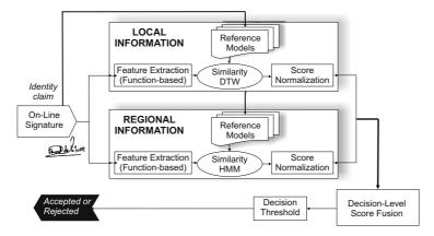
Fig. 1. System model of multilevel signature verification
