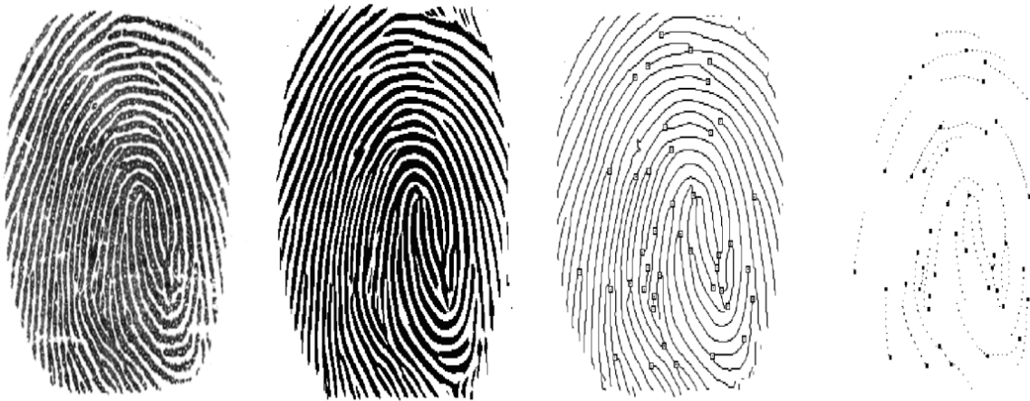
Figure 7.2: Processing steps of the minutiae-based matcher.
