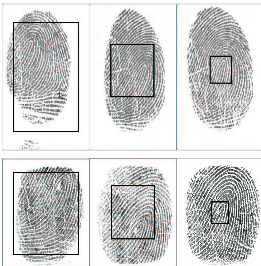
Figure 4.3: Three impressions belonging to a given finger, acquired both with the optical scanner (top) and the capacitive scanner (bottom) under the three levels of control considered in the MCYTDB fingerprint corpus (from left to right).
