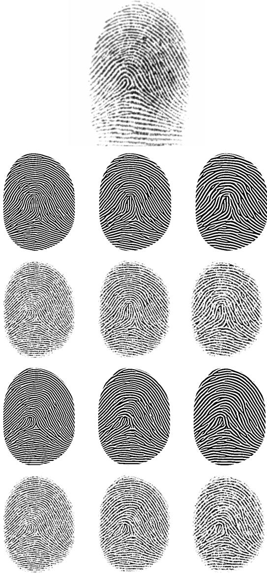
**Figure 3:** A fingerprint and all the images reconstructed from its template in the various experiments. From top to bottom: MinTYPE-BIN, MinTYPE-REN, ORIMG-BIN, and ORIMG-REN. From left to right: ridge-line period = 7, 8, 9 pixels.
