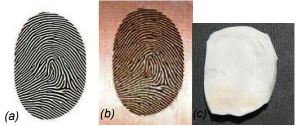
**Figure 2:** Reconstructed fingerprint image (a), fingerprint printed on the PCB (b), fake silicon fingertip (c).
