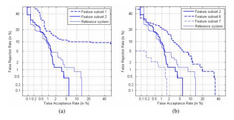
**Fig. 4.** (a) Performance obtained using three different feature sets. This experiment reports results about which fingers must be included in the feature set. (b) DET comparative between four proposed feature sets. In this picture, the influence of palm and finger widths is examined.
