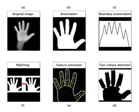
**Fig. 1.** Block diagram of the main steps followed in our system to extract features and matching two hands. Original image (a) is first binarized (b). The boundary is then calculated and the plot (c) of the radial distance from a reference point lets us estimate the coordinates of tips and valleys (d). After that, feature extraction is done by measuring some finger lengths and widths (e). Last, given two hands, their matching is based on a distance between their feature sets.
