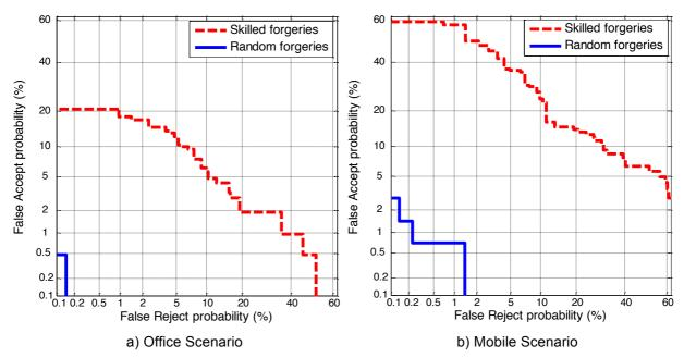
Figure 5. DET curves results for the two operational scenarios considered in this study, showing for each case both skilled and random forgeries results.
