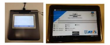
Figure 2. Devices used in this study to acquire dynamic signatures. Left, Wacom STU-530, and right, Samsung Galaxy Note 10.1.
