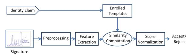
Figure 1. Arquitecture of a dynamic signature verification system.
