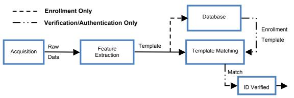
Figure 2. Block diagram of biometric authentication systems
