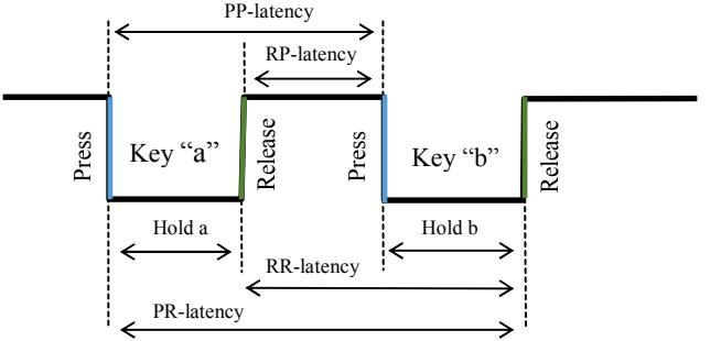
**Figure 2:** Keystroke dynamics features from a digraphs sequence.
