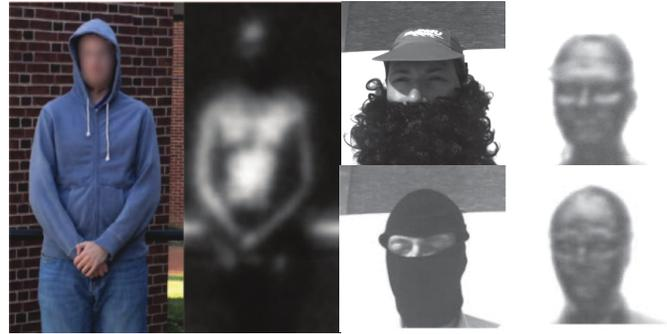
Fig. 2. Benefits of mmWs for imaging: *i*) transparency through body clothes (extracted from [3], and *ii*) transparency through face clutter (images from the mmW TNO database).
