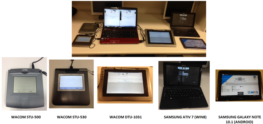
Fig. 1. Acquisition setup for e-BioSign database.
