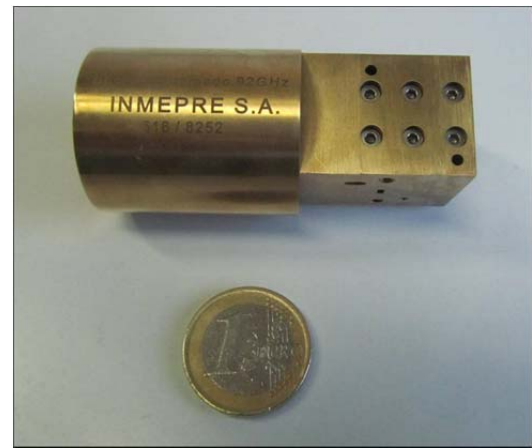
Fig. 33. Circular Polarization Waveguide Duplexer (Horn + Septum-OMT) at 100 and 225 GHz
