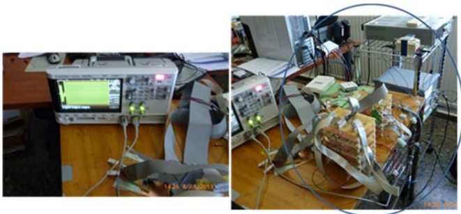
Fig. 27. LC Switching Time Measurement Setup
