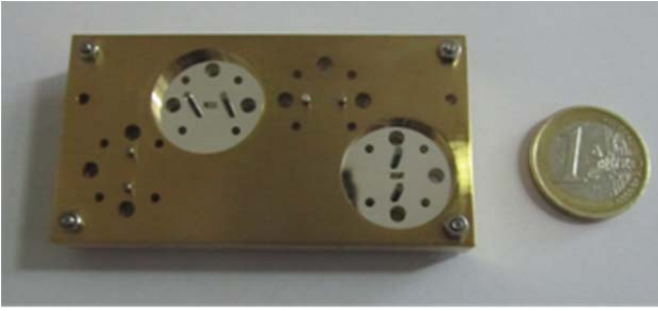
Fig. 35. Dual-band SU-8 Micromachined OMTs
