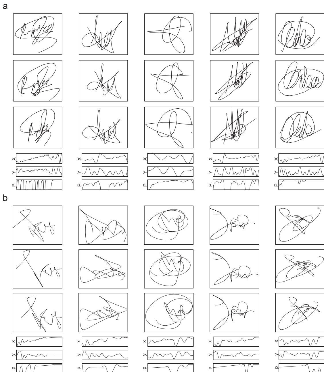
Fig. 8. Examples of real (a) and synthetic (b) signatures extracted from MCYT and SDB1, SDB2. Three samples of five different real and synthetic signers are shown together with the time sequences x[n] , y[n] , and p[n] corresponding to the first sample. (a) Real signatures extracted from the MCYT database [85]. (b) Synthetic signatures produced with the proposed model-based generation algorithm.
